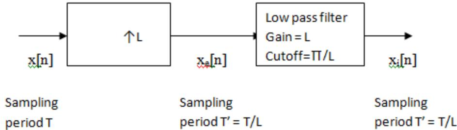
Fig 1 General system for sampling rate increase by  $L$ .
